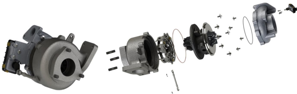
Fig. 3 – Disassembled component – a turbocharger. Source: own research
